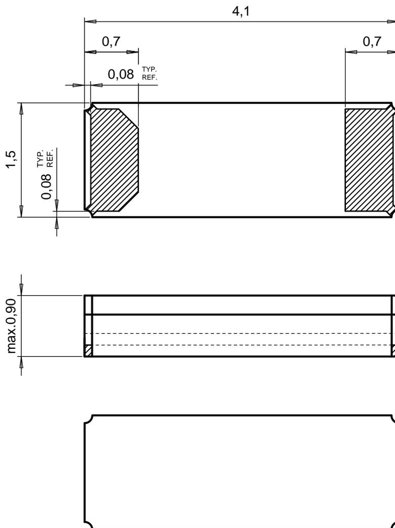
Tolerances: unless otherwise specified  $\pm 0.1\text{mm}$
