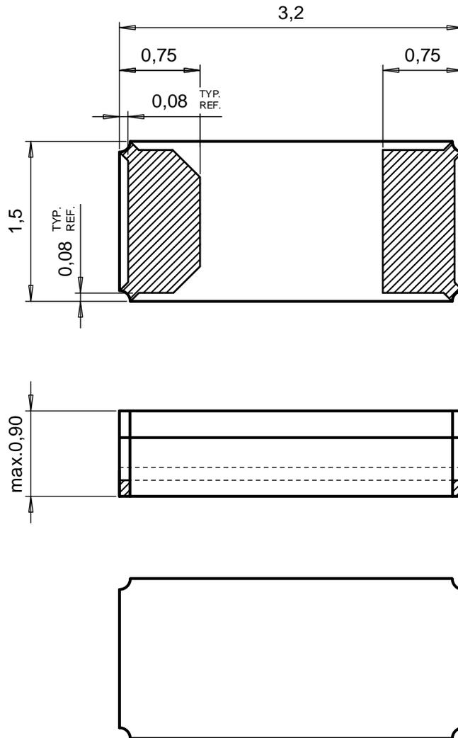
Tolerances: unless otherwise specified  $\pm 0.1\text{mm}$
