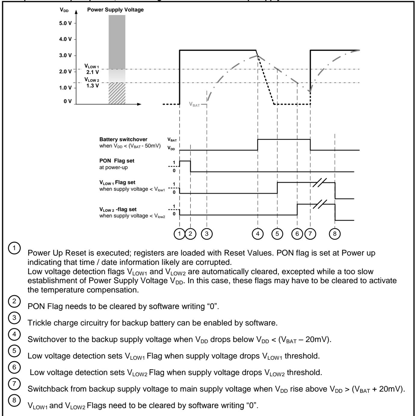
**4.1.2.SUPPLY VOLTAGE OPERATING RANGE AND LOW VOLTAGE DETECTION**
