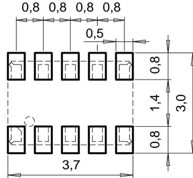
Metal lid is connected to  $V_{SS}$  (pin #6)
