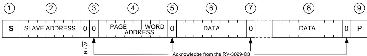
**6.8.2.READ MODE DATA TRANSMISSION AT SPECIFIC ADDRESS**
