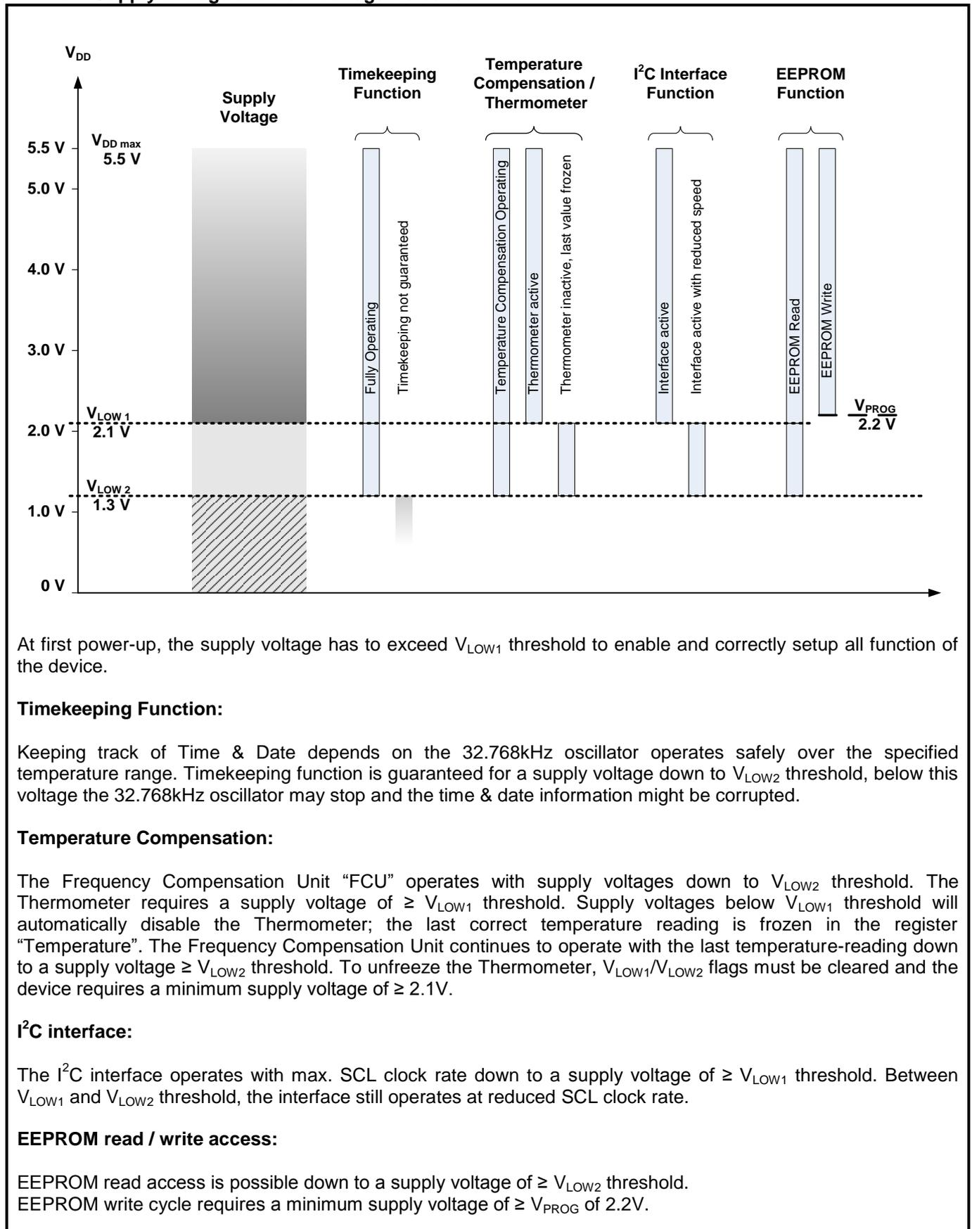
At first power-up, the supply voltage has to exceed  $V_{LOW1}$  threshold to enable and correctly setup all function of the device.
