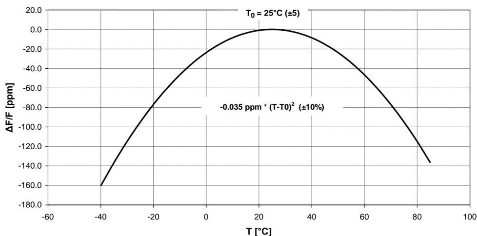
Above graph shows the typical frequency-deviation of a 32.768kHz "Tuning-Fork" Crystal over temperature. The parabolic curve is specified in terms of turnover temperature " $T_0$ " and the quadratic thermal coefficient " $\beta$ ".
