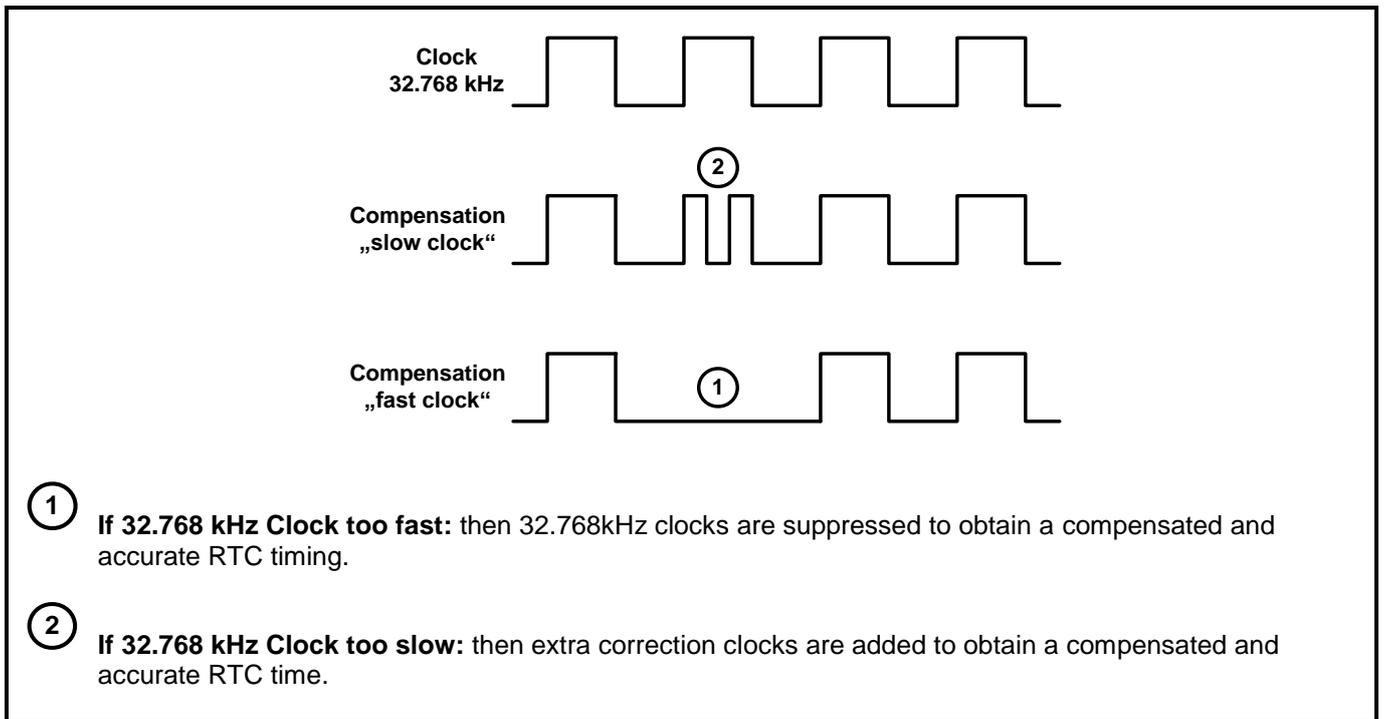
Each compensation period takes 32 seconds. Correction clocks are periodically applied during one complete compensation period. Within a compensation period of 32 seconds, one correction clock will compensate the time information by  $\pm 1$  ppm.
